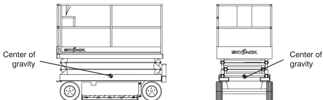
Figure 3-15. Center of Gravity
